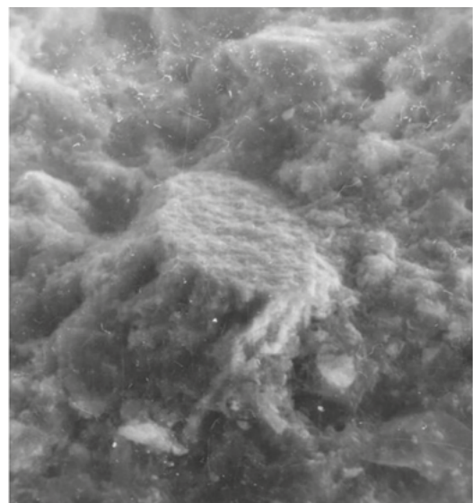
Figure 8 – Micrographs of a cement stone based on a modified binder after exposure to \gamma -radiation with a dose of 10^9 rad
