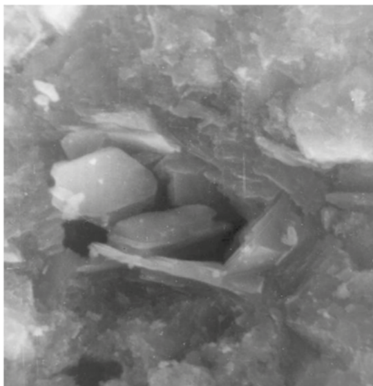
Figure 7 – Micrographs of cement stone based on Portland cement after the action of \gamma -radiation with a dose of 10^9 rad
