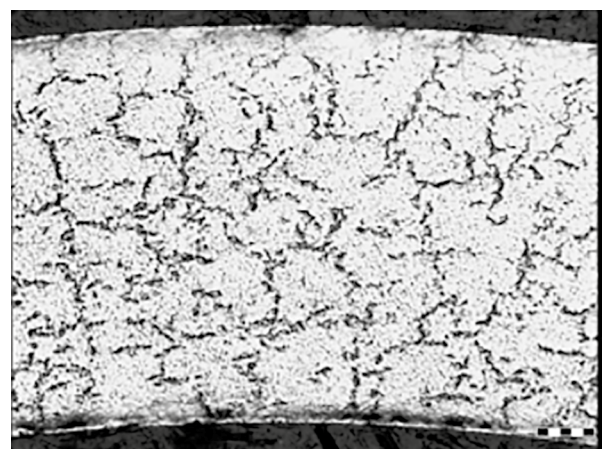
Figure 4 – Sample No 48: 400 ppm, P_{293} = 5.0 MPa, 3 thermal cycles 410 \leftrightarrow 300 °C, F_n \approx 0.96
