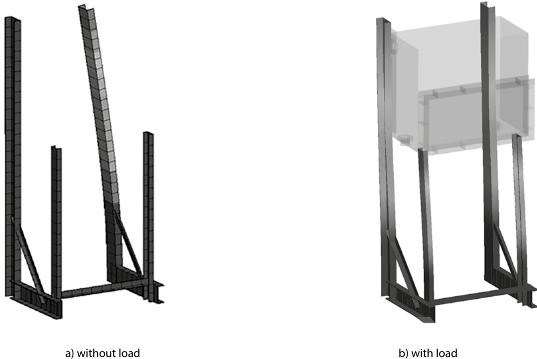
Figure 7 – The first mode of support structure natural frequencies for the without load and with load cases
