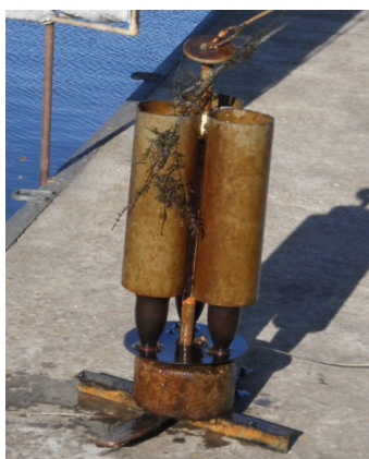
Fig. 1. Set of vertical sediment traps on the pier of the State Institution "Scientific Hydrophysical Center of the NAS of Ukraine"
