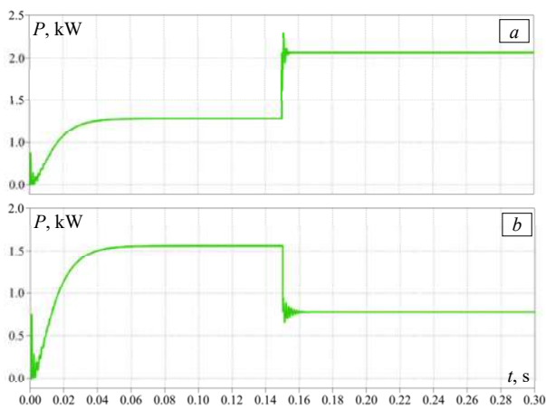
Fig. 18. AC load at t = 0.15 s for case 1: a – AC load increase 610 W; b – AC load decrease 750 W
