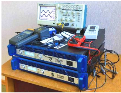
Fig. 8. Power amplifiers for powering the active shield compensation windings
