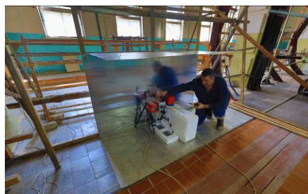
Fig. 4. Solid passive shield without side plates
