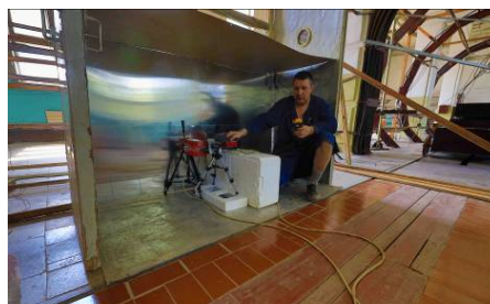
Fig. 5. Solid passive shield with side plates on either side of the shield
