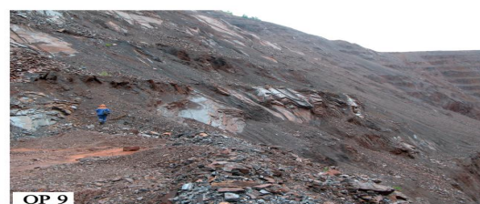
Fig. 1. Photo of structural elements of technogenic embankments (OP 0) and outcrops of pillars among unstructured scree in the eastern side (OP 9) of the “Pivnichnyi” quarry.
