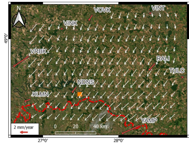
Fig 3. Annual station velocities and condensed vector field of GNSS stations around the Dnister Hydropower Complex.
