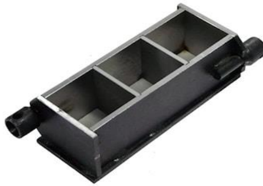
Figure 1– Metal mold (3FK-100) for manufacturing cubic samples of CSM with a face size of 100 mm
